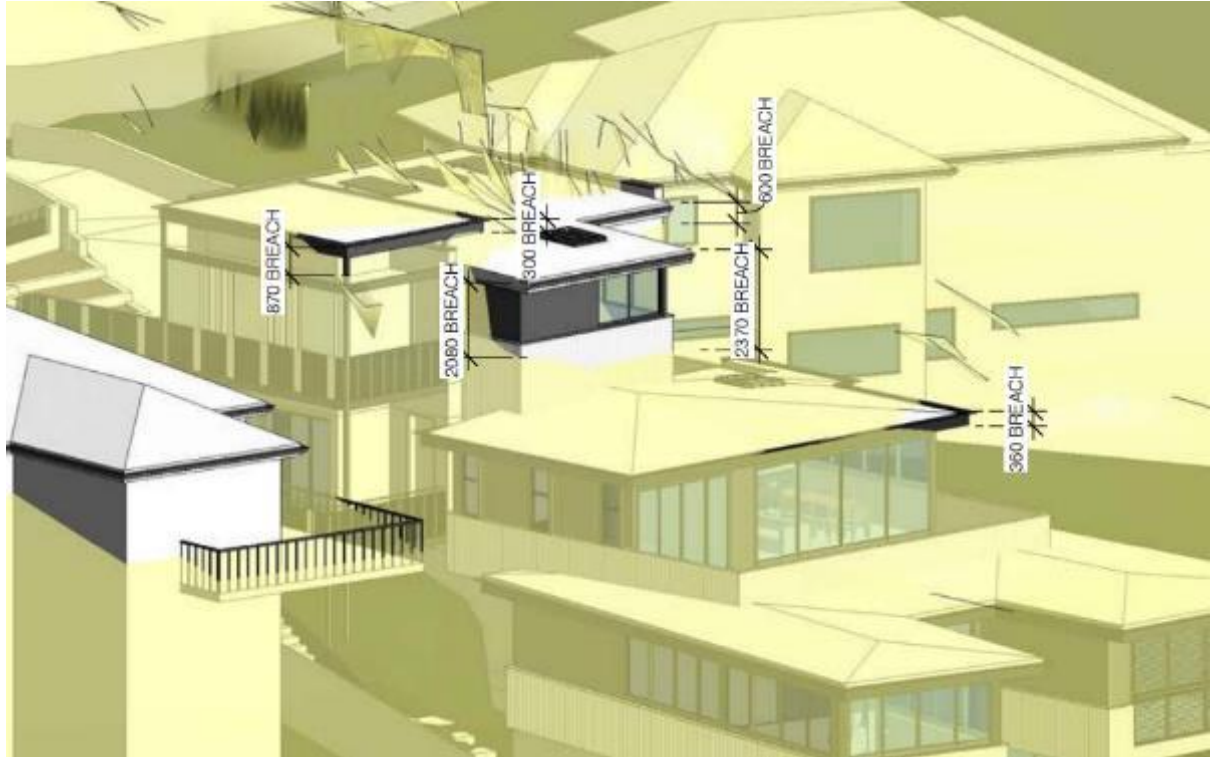
Figure 1 - Building height plane blanket (in yellow) showing the breaching elements above the 8.5 metre height standard.
